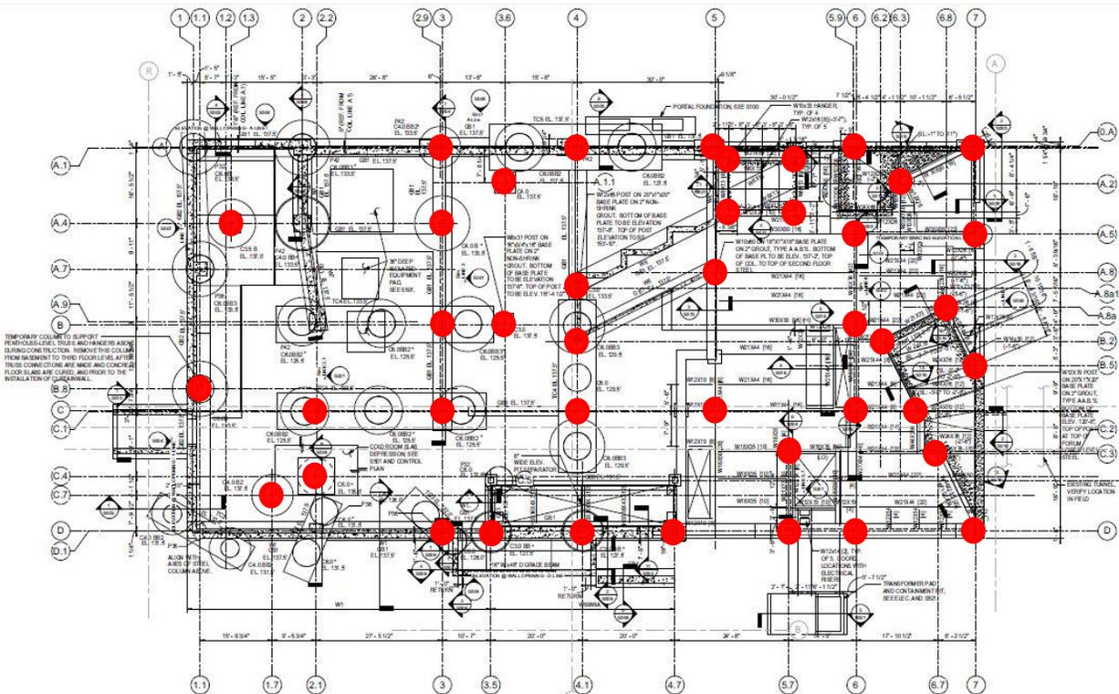
**Figure 6** – Column Layout (Highlighted in Red) for the Basement Level
