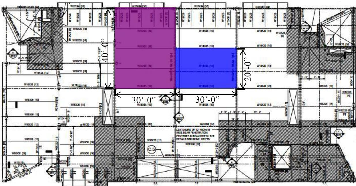
Figure 7 – Typical Floor Plan with Typical Bay Sizes Emphasized
