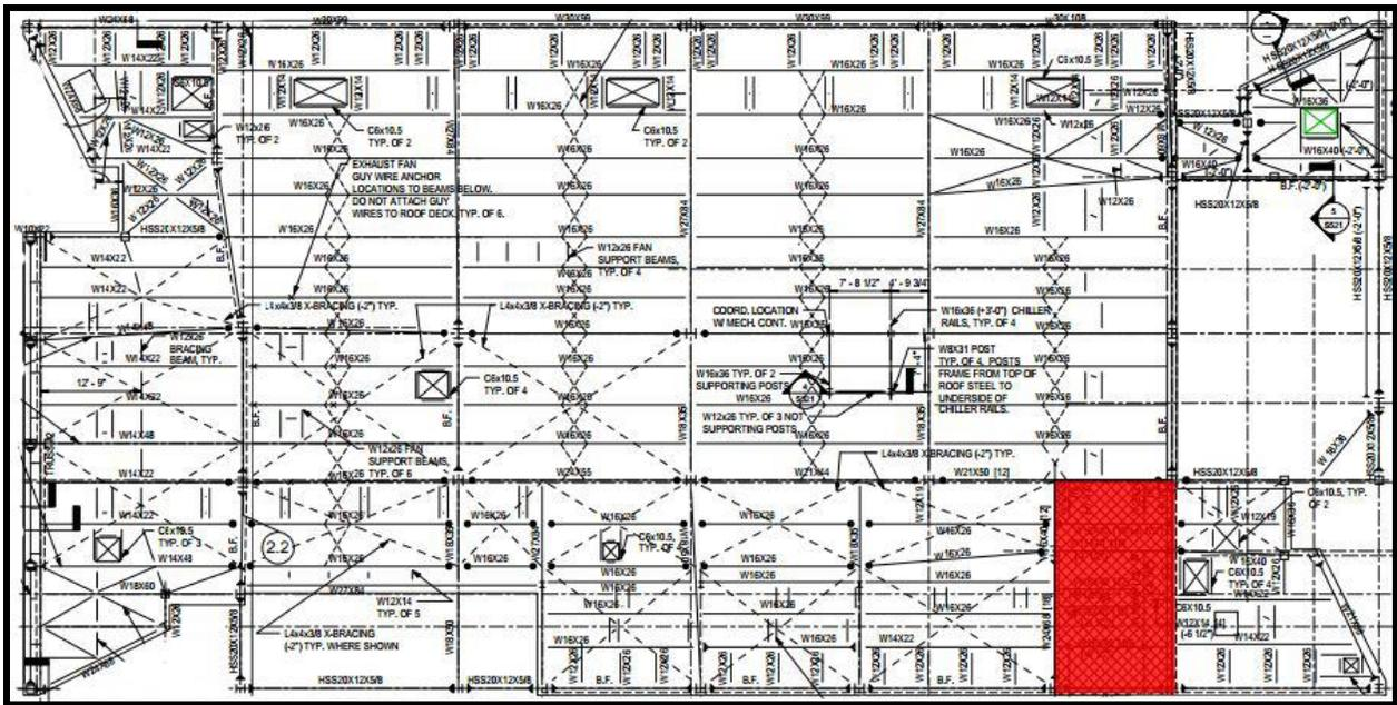
Figure 9 – Roof Framing Plan with Added Concrete Slab-On-Deck Highlighted
