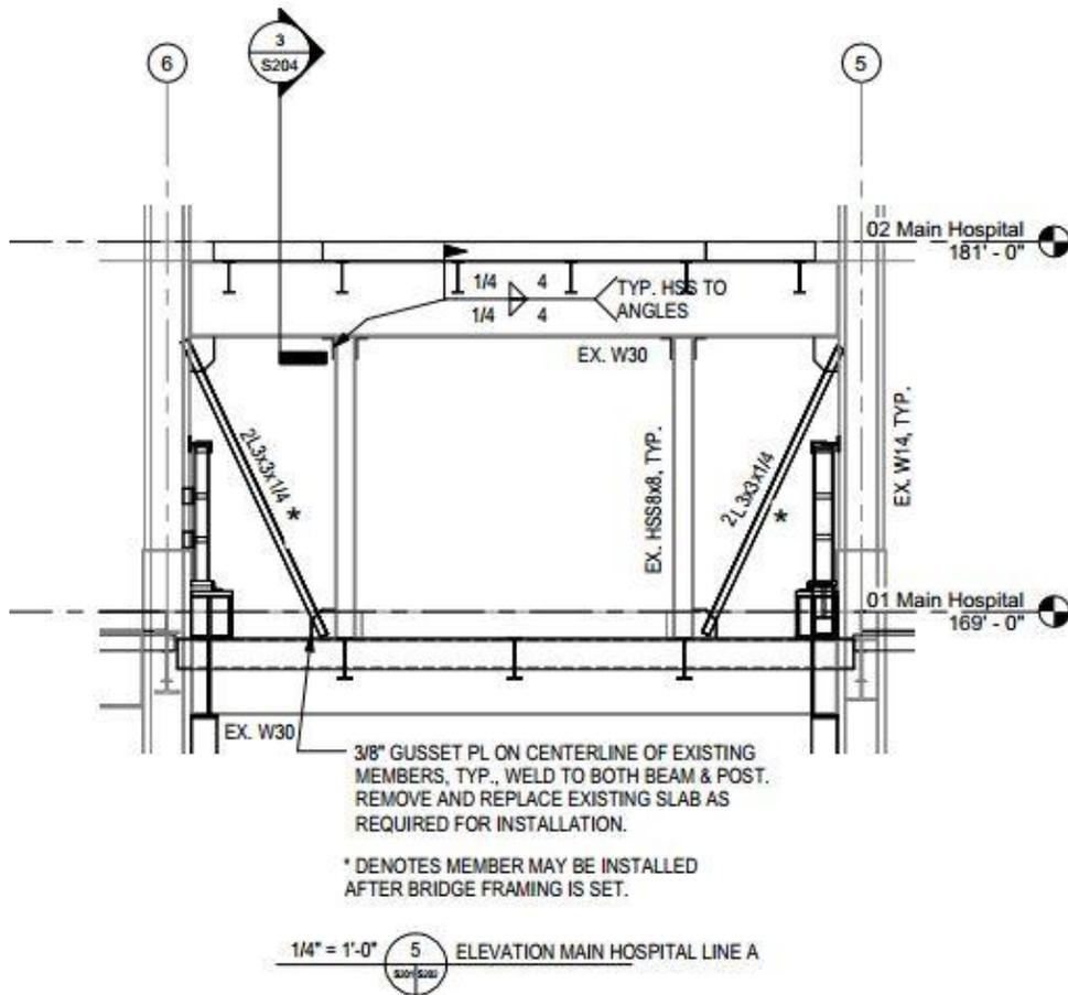
**Figure 11** – Elevation of Bridge Connection with Main Hospital
