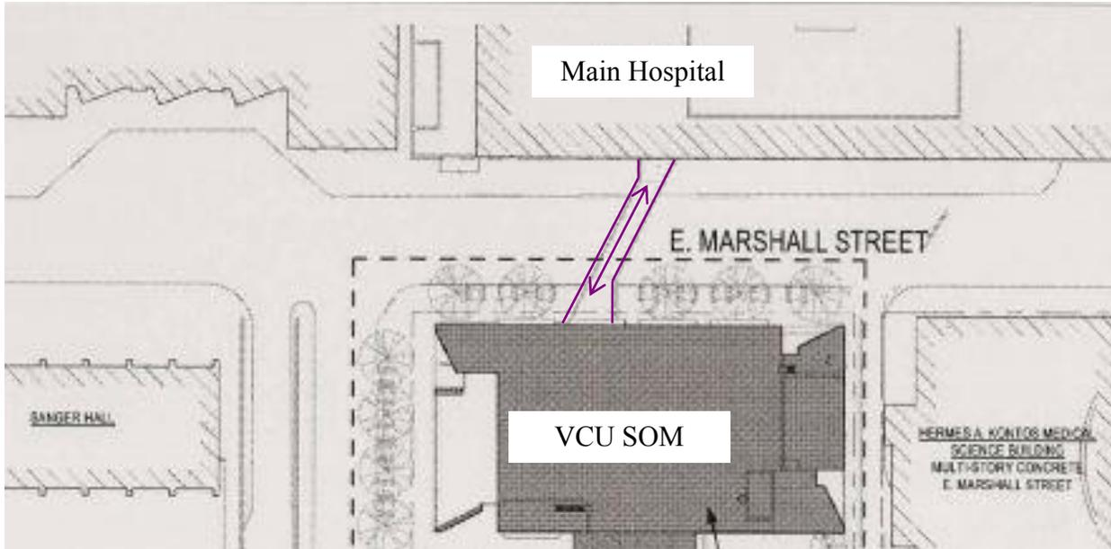
**Figure 10** – Bridge Connecting VCU SOM to Main Hospital
