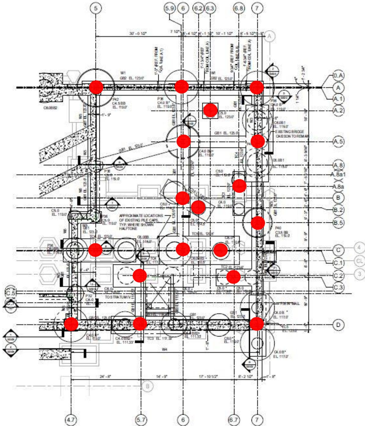
Figure 4 – Column Layout (Highlighted in Red) for the Sub-Basement Level
