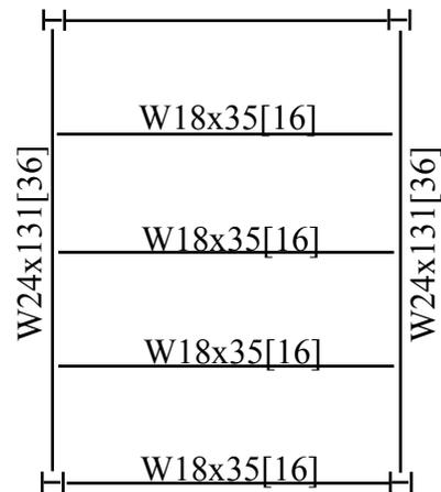
Figure 9 – Detailed Drawing of “Larger” Bay
