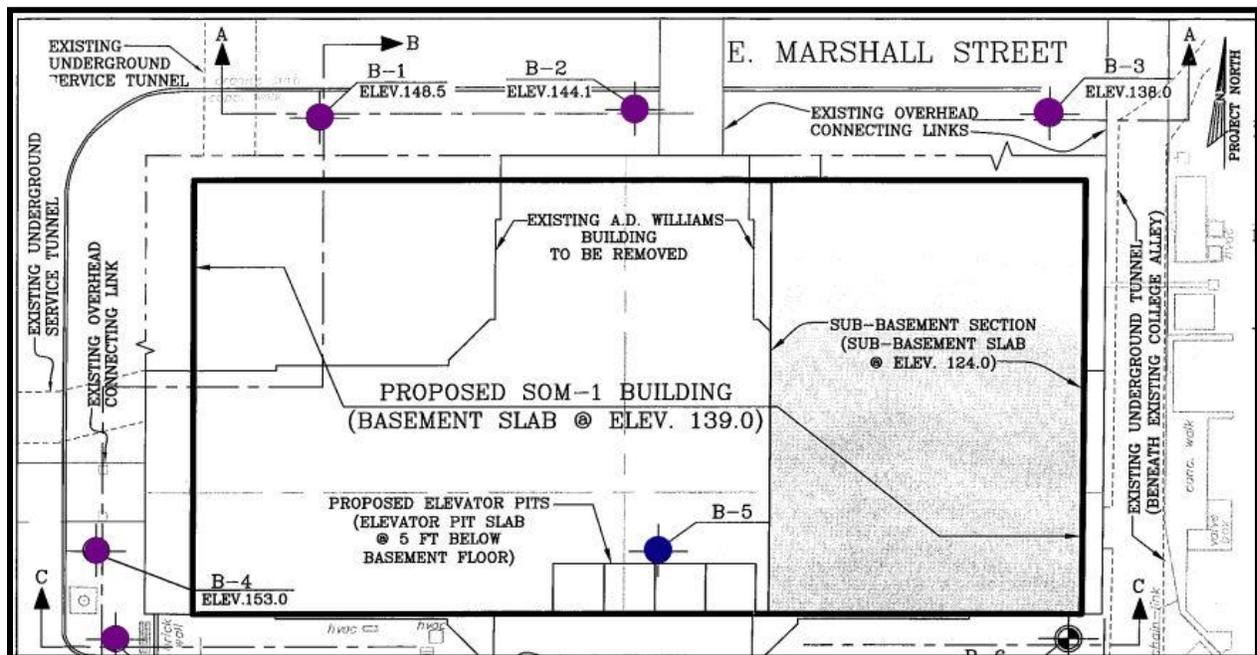
*Figure 2* – Test boring sites, highlighted in color, established in the field by Geotech, Inc.
